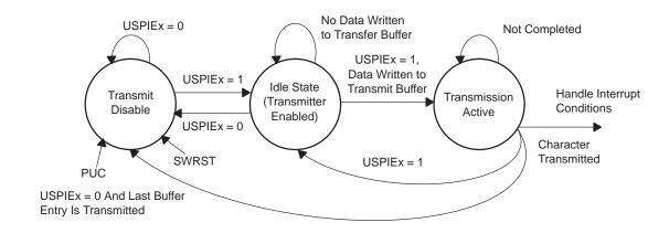
Figure 14-5. Slave Transmit Enable State Diagram
